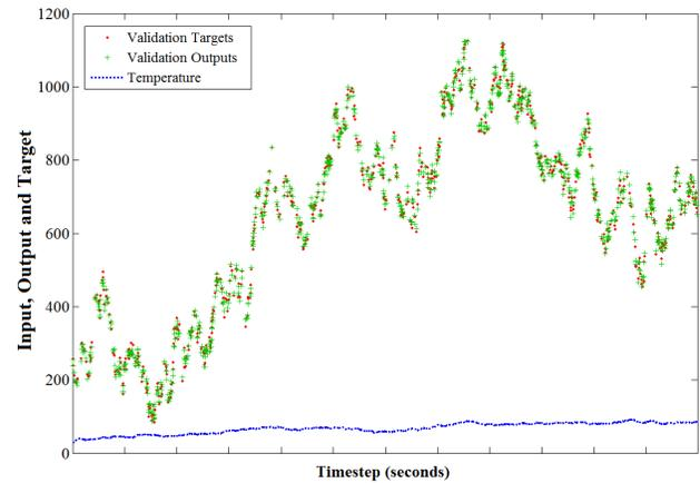
Fig. 8. Prediction performance of best-performance NARX model with a 7-second delay input data from Table I (c) representing an induction motor/surface overheating situation
