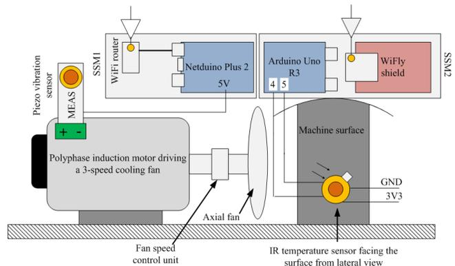
Fig. 2. Architecture of the mechanical test-bed based on two smart sensor modules measuring serial vibration and temperature data transmitted via a TCP/IP socket connection to the CCU
