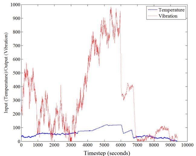
Fig. 4. Training data representing the time-series response showing outcome vibration pattern against artificially induced temperature changes (temperature shown as the lower data with changes induced from frame 3000 – 6500)
