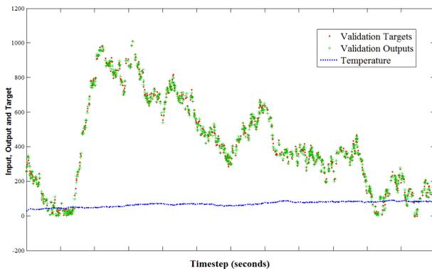
Fig. 7. Prediction outcome of best-performance NARX model with a 7-second delay input data taken from situation given in Table I (d) representing an erratic (induced) fan failure condition
