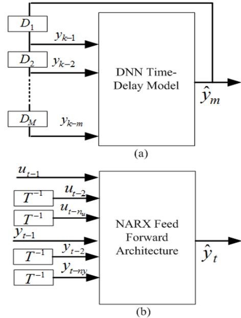
Fig. 3. (a) A DNN network without exogenous data and (b) a series-parallel NARX architecture where -  $u$  is the exogenous (temperature) input and  $y$  is the autoregressive vibration variable and  $\hat{y}$  corresponds to the classification of the autoregressive variable
