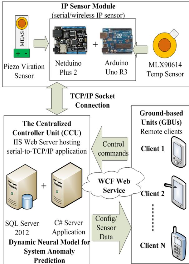
Fig. 1. The three-tier, embedded client-server architecture based on dynamic neural network modeling for condition monitoring
